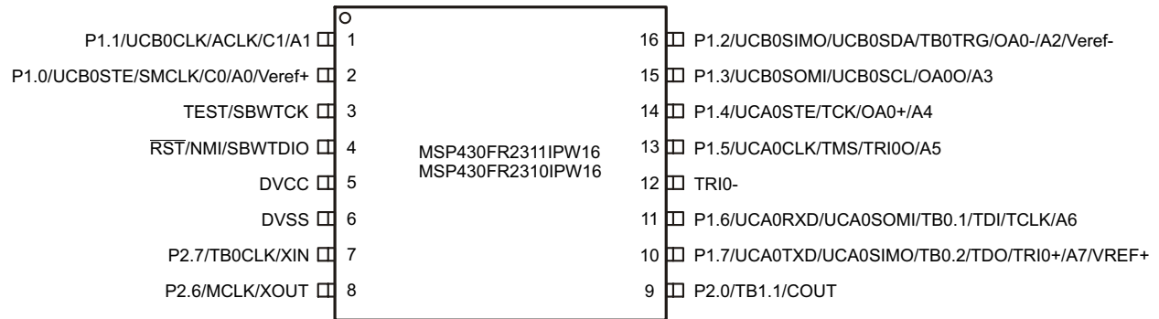
Figure 4-3. 16-Pin PW (TSSOP) (Top View)
